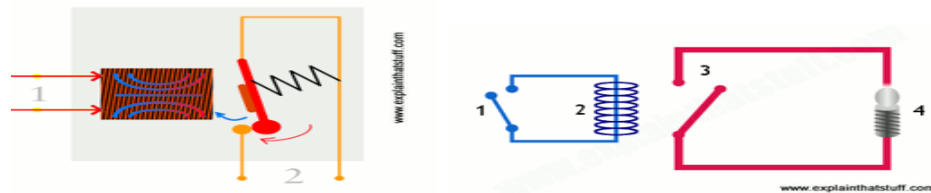
Figure6: Working principle of relays
