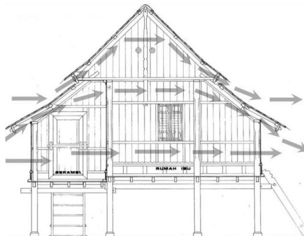
Fig. 2: Ventilation Openings in the Roof of Traditional Malay House
