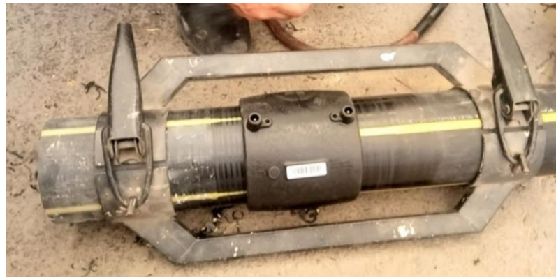
Figure 8: Welded coupling after initial cooling period before submersion in ice water bath;
