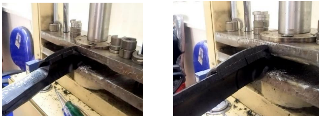
b) application of compression force to the second part of the sample coupling a) application of compression force to the first part of a coupling
