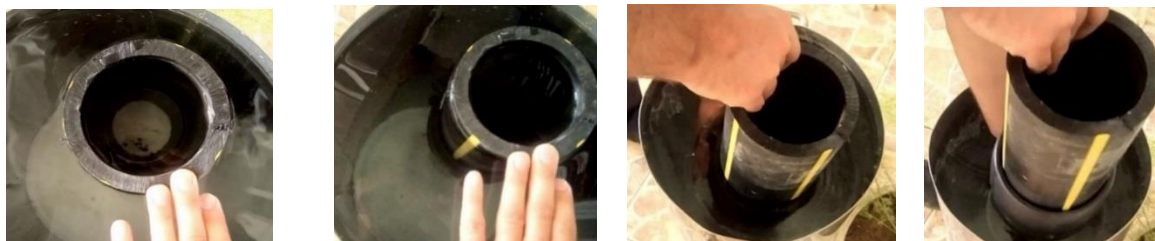
b) stabilization of the coupling in the ice water bath
