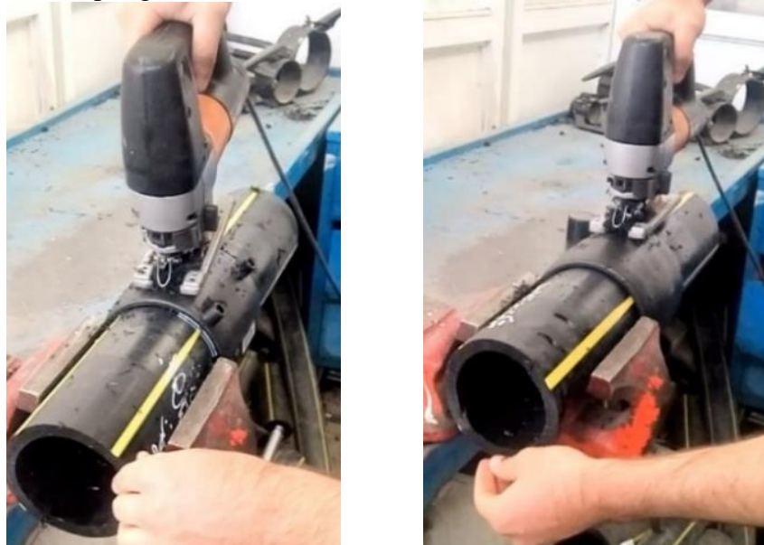
Figure 10: Cutting of the coupling after final cooling for crush test
